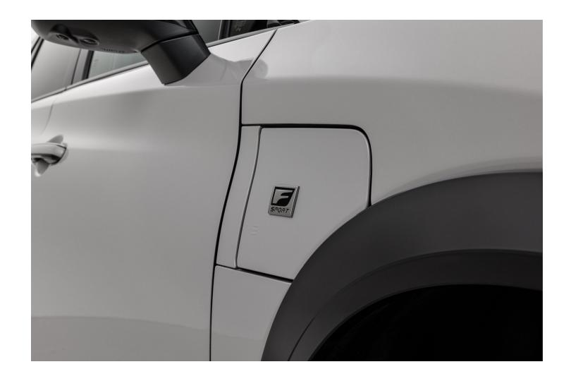
The 2026 RZ adopts the North American Charging System (NACS) charging port (SAE J3400) on the passenger's side of the vehicle, enabling access to thousands of high-speed charging stations nationwide. It also has Level One and Level Two AC charging with a higher-capacity 11-kW on-board AC charger (up from 7-kW capacity on the prior model year).
